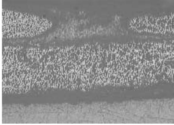
Figure 1: A real micrograph of a transverse plane section of the fiber tow
