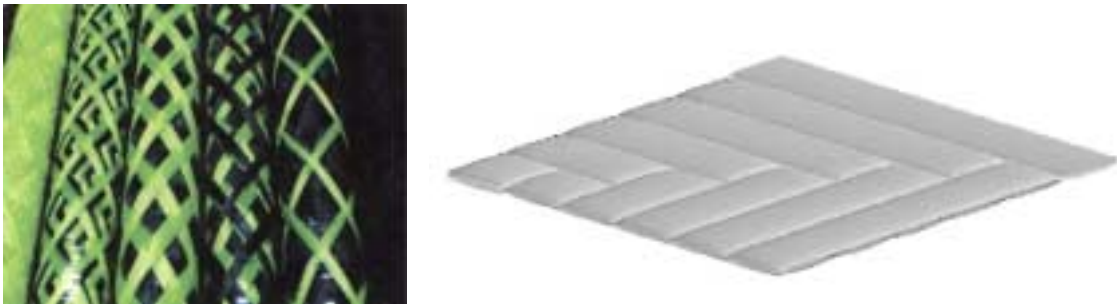
Figure 7: Modeling on meso-scale: tube sample and periodic unit cell model
